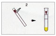
2. Remove the NicCheck test strip from its container using a gloved hand or forceps. Insert the strip, arrow pointing downward into the tube containing urine. NOTE: Under humid conditions, stopper the tube.
